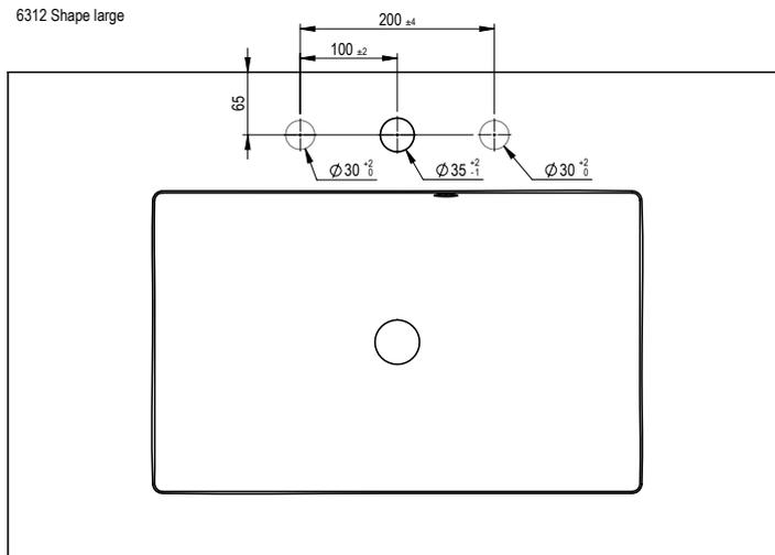
3-holes fixtures holes for Shape and Form to cabinets with a depth of 400 mm
